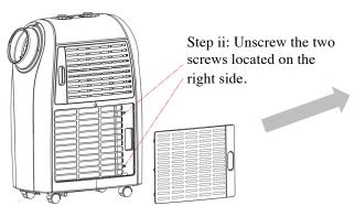
Step i: Remove the filter by gently pulling it out.
