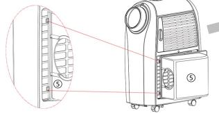
Step iii: Attach the hood by aligning it with the unit. Be cautious of the two inserts on the left side and carefully slide them in.
